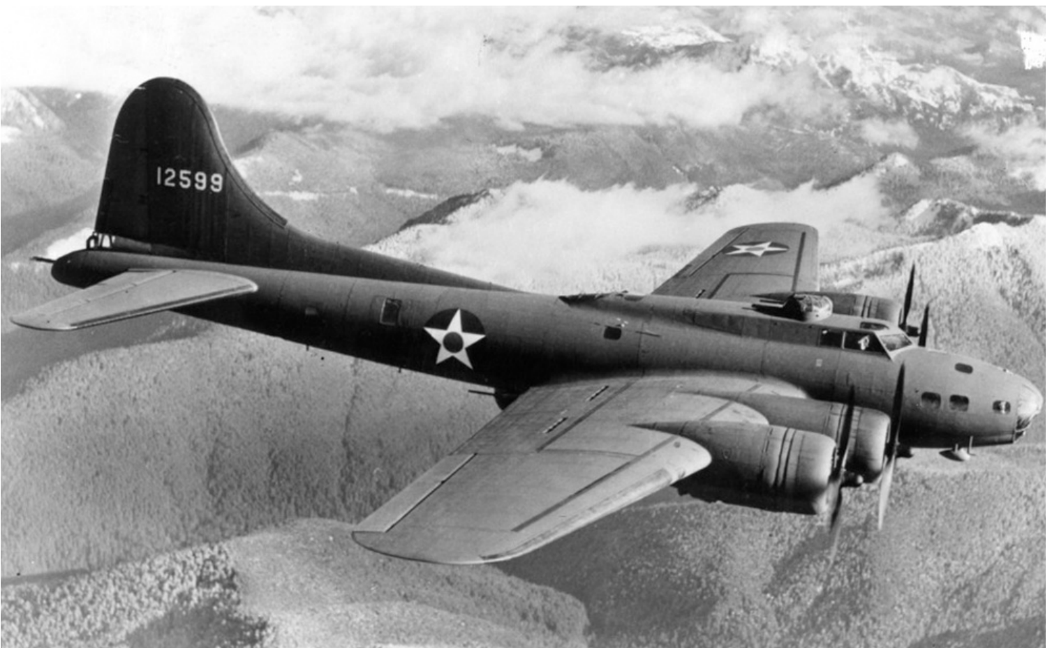
The B-17E, the first mass-produced model of the Flying Fortress, carried nine machine guns and a 4,000-pound bomb load. It was several tons heavier than the prototypes and bristled with armament. It was the first Boeing airplane with the distinctive — and enormous — tail for improved control and stability during high-altitude bombing.
